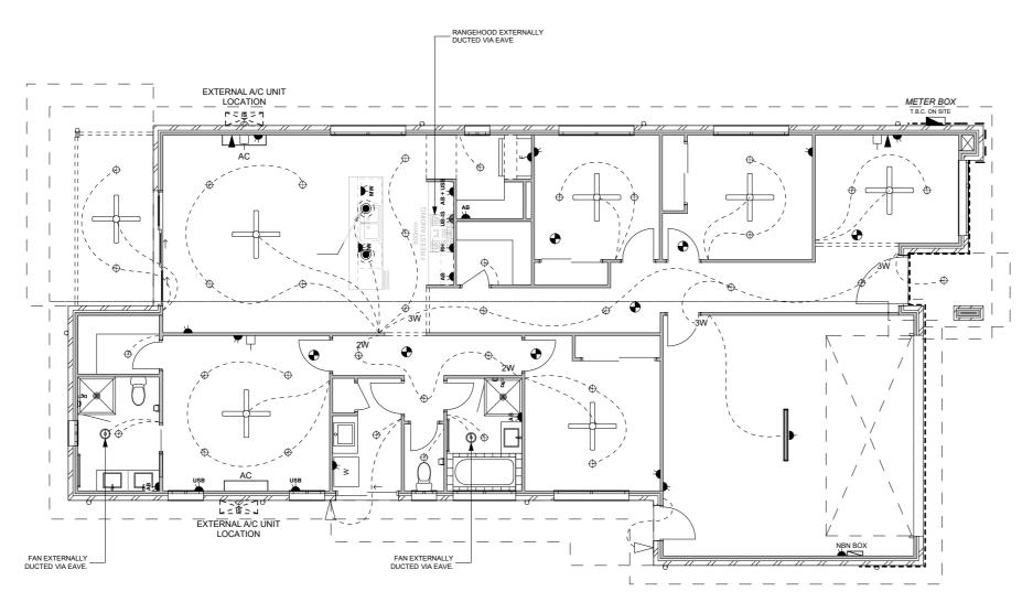
NOTE:-KITCHEN RANGEHOOD, BATHROOM AND ENS EXHAUST SYSTEMS TO BE EXTERNALLY DUCTED VIA EAVES.
